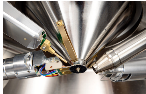
A look inside the chamber with the annular BSE detector (aBSD) mounted under the pole piece of the objective lens enabling imaging in variable pressure (NanoVP lite mode) and 3D surface modelling (3DSM).
