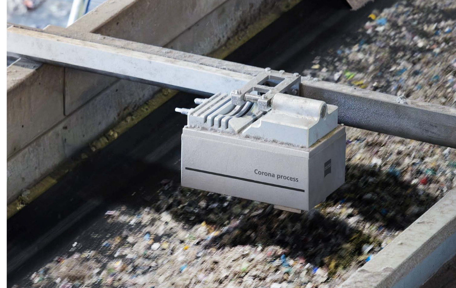
Corona® process mounted over conveyor belt
