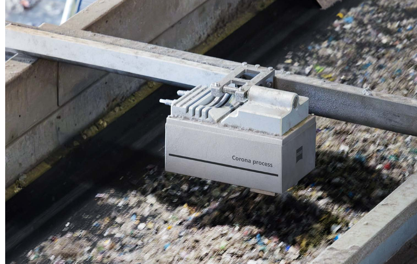
Corona® process mounted over conveyor belt
