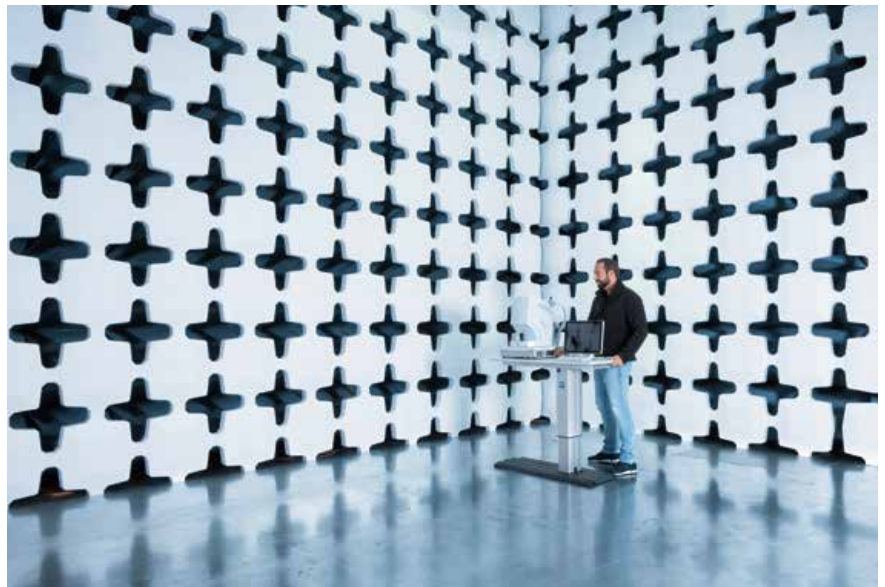
Standard-compliant testing of medical electrical equipment. Anechoic chamber with 10 m measurement range.
