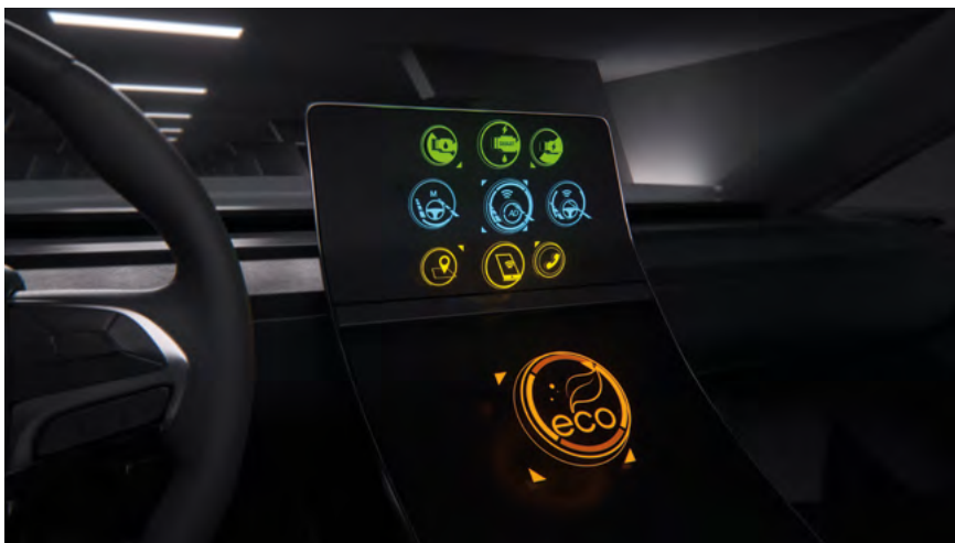
FIGURE 4 An example of holographic switches as an alternative to conventional 3-D control elements: They can be activated by voice commands or gesture control for example (© Zeiss)
