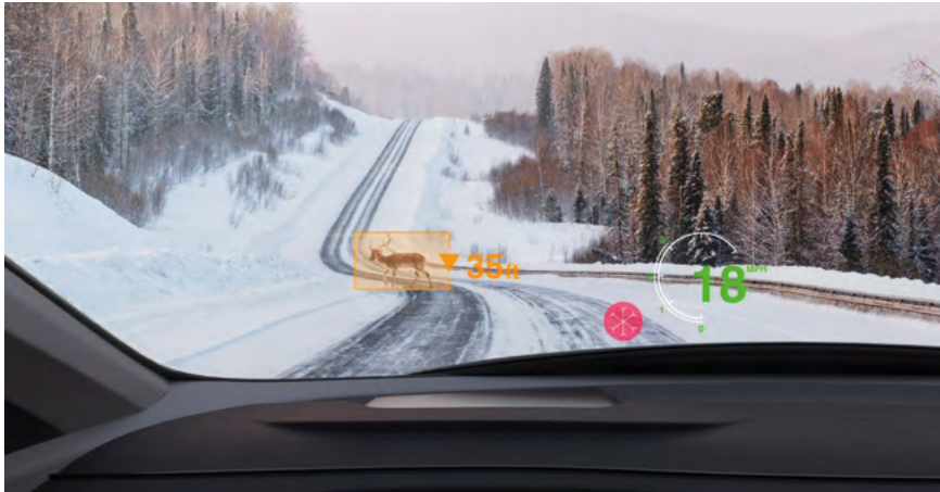
FIGURE 3 Warning symbols or emojis can be fully customized – even in rear and side windows; it is also conceivable to incorporate information on points of interest, restaurants or events; video content can be displayed (© Zeiss)
